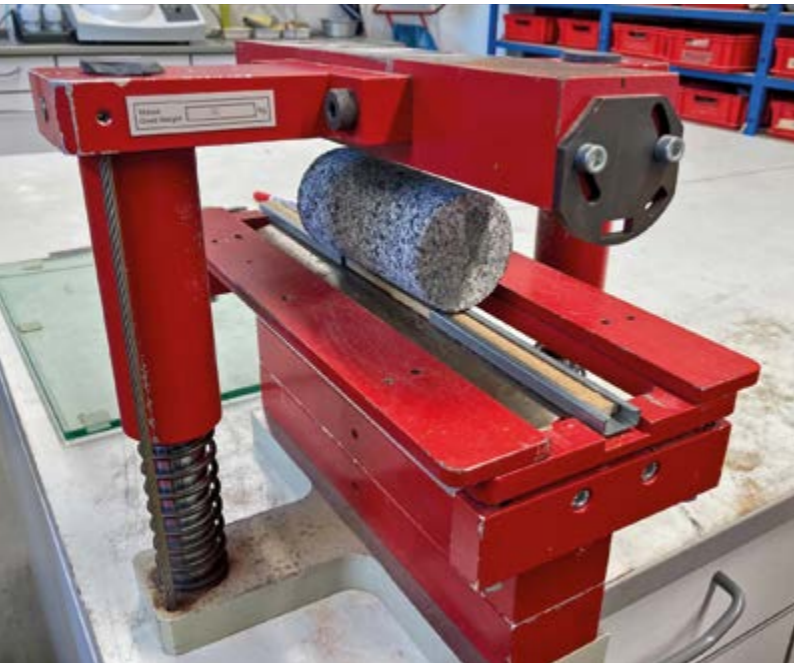
Such rock samples – whether from stock or newly taken – are tested for their behaviour under high pressures.
